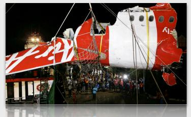
said that a solder joint in a circuit board could have led to rudder problems that caused the crew to try to fix the autopilot by re-setting a circuit breaker. The crew eventually lost complete control of the airplane.
